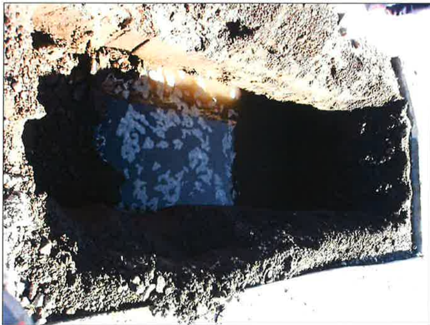
Photo 4: Groundwater Seepage and Gravel Deposits Cave-In in TP8
